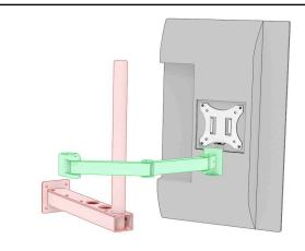
The screws, M6 Philips type, for fixing the arm to the table are already fitted to the table. Remove them from the table on the side you would like to fit the monitor then use them to secure the arm to the table as shown here.
